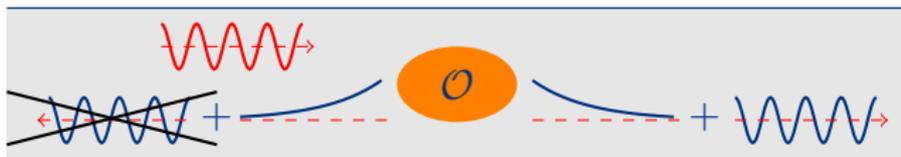
The idea is to use a **complex scaling** (and numerically **PMLs**), with complex **conjugate** parameters at both sides of the obstacle, so that the transformed  $u$  will belong to  $L^2(\Omega)$ .
