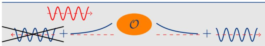
The idea is to use a **complex scaling** (and numerically **PMLs**), with complex **conjugate** parameters at both sides of the obstacle, so that the transformed **total field**  $u$  will belong to  $L^2(\Omega)$ .
